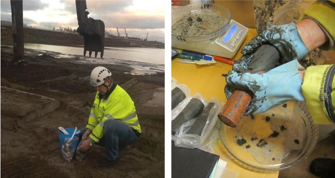
Figure 10. Sampling for environmental eligibility testing during stabilization works (left) and making of test specimens (right).
