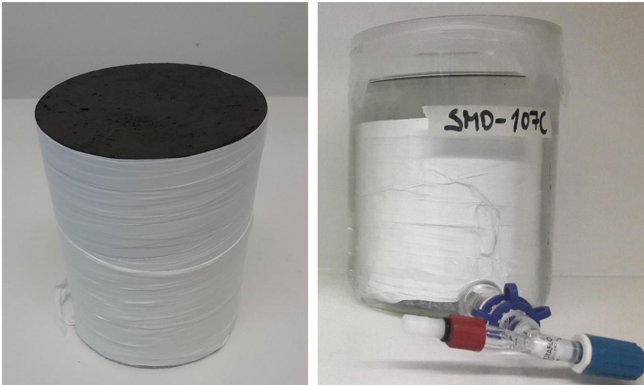
Figure 3. Prepared stabilized test specimen (left) and submerged stabilized test specimen (right) during surface leaching test.
