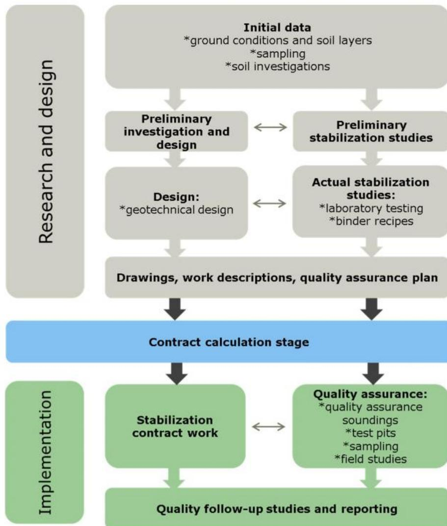
Figure 1. Main phases of mass stabilization project (Ramboll Finland Oy, 2015).
